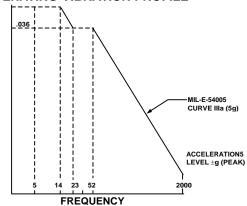
CURVE IIIa - EQUIPMENT MOUNTED FORWARD HALF OF FUSELAGE 5 OR IN WING AREA WITH ENGINES AT REAR OF FUSELAGE
